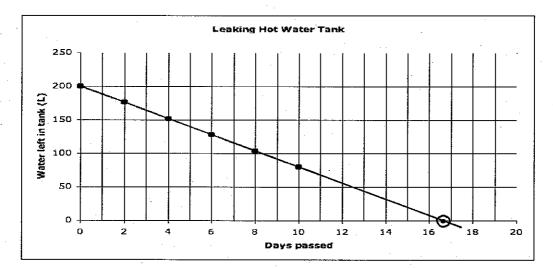
Extend the line to determine how many days must pass until the tank is empty. ANS 17 days.
